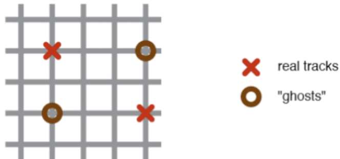
Figure 2.18: Two real tracks forming two ghost hits in a 2D-microstrip detector.
