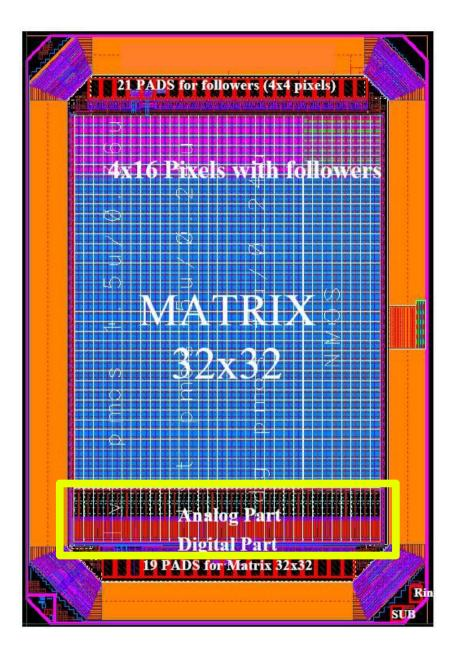
Analog and digital circuits are built in the <u>chip periphery</u> and <u>integrated</u> on the same sensor silicone die !
