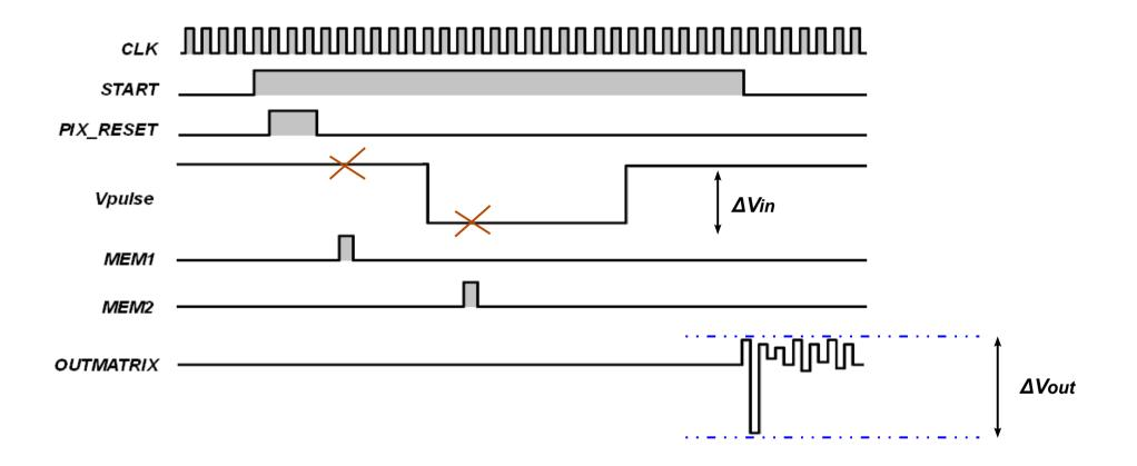
total gain (sensor + electronics) =  $\Delta Vout / \Delta Vin$
