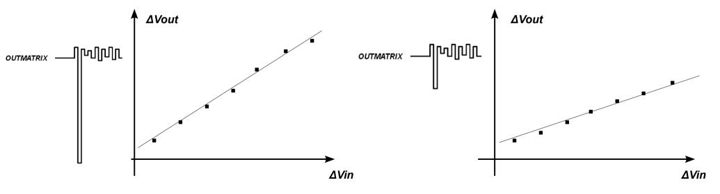
read-out voltage gain =  $\Delta Vout / \Delta vin \rightarrow liner fit slope$
