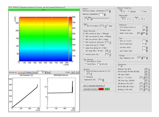
The two plots at the bottom of the "Drift potential" tab show: a. drift potential along the y coordinate (calculated on strips or between strips, according to the option "Plotting at". By default it is calculated at the middle of the central electrode, but is selectable from number entry); b. drift field along y or x
