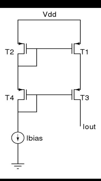
$r_{out1} \approx g_{m3} r_{03} r_{01} \approx 20 M \Omega$
