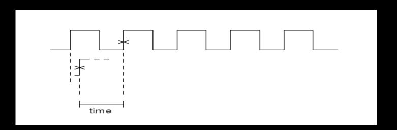
Since the rate per strip is about 30 kHz the biggest signal is exhausted in 3.2us, so we have a pile-up problem. We want a system that has 1LSB = 400ps
