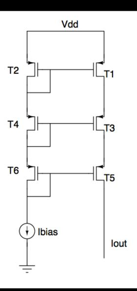
$$r_{out} \approx g_{m5} r_{05} r_{out1} = g_{m5} r_{05} g_{m3} r_{03} r_{01} \approx 550 M\Omega$$
