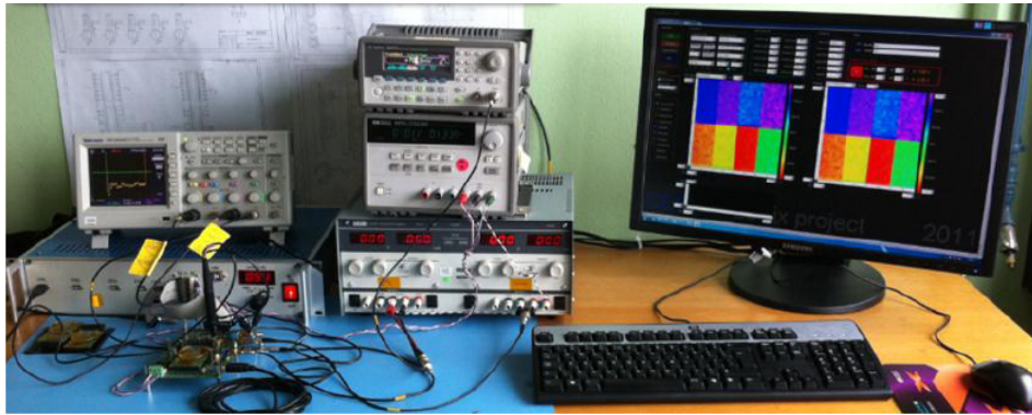
Figure 6.18: Experimental equipment used to test the LePix matrix: in the bottom part on the left it is possible to see the DAQ box and the boards, in the central part the power supplies used to bias the chip and on the right the online view with the matrix sectors.
