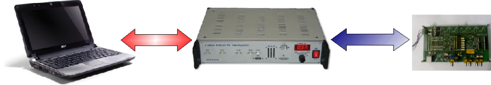
Figure 6.17: Schematic view of the I/O communications: the ROOT based software allows to set the timing of the signals sent by the DAQ to the boards; then the signals at the output of the boards are elaborated by the DAQ to be saved by the software.
